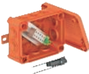
T 100 ED 6-6 AF with external fastening with 6 terminals for cables with a nominal cross-section of 6 mm 2 and fuse holder TE-FH 520 Item no. 7205560
