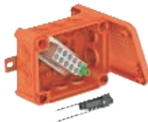
T 100 ED 10-6 AF with external fastening with 6 terminals for cables with a nominal cross-section of 10 mm 2 and fuse holder TE-FH 520 Item no. 7205563
